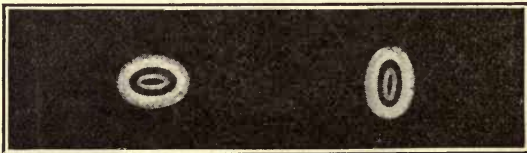
FIG. 163. FIG. 164. FIG. 163.—Astigmatism Inside Focus. FIG. 164.—Astigmatism Outside Focus.
